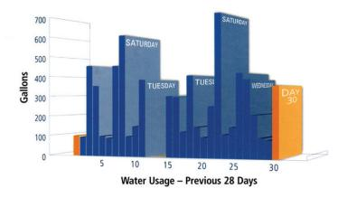
The patented microprocessor keeps a running average of the previous 28 days of water usage and automatically adjusts to your family's requirements
